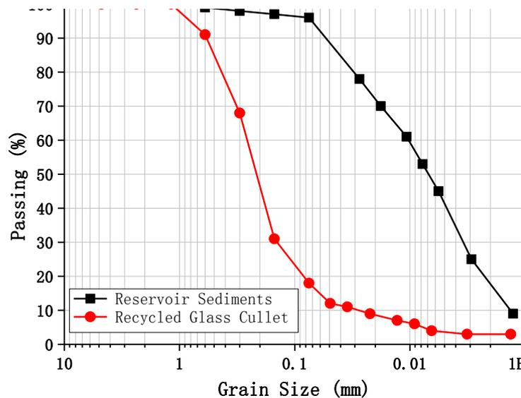
Fig. 1 Grain size distributions of cullet and reservoir sediments
