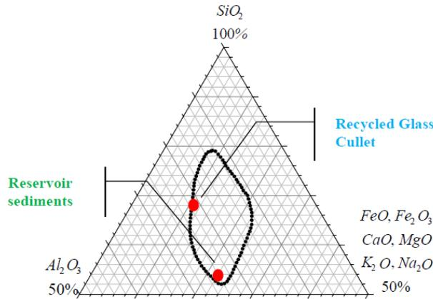
Fig. 2 Ternary diagram of cullet and reservoir sediments
