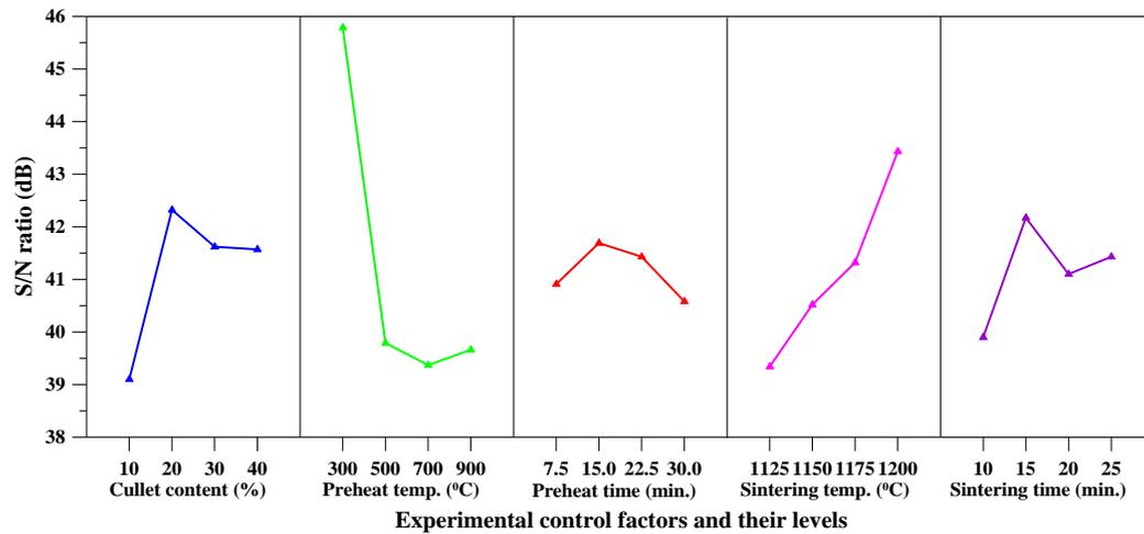
Fig. 5 S/N response graph for bloating ratio
