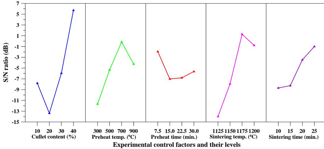
Fig. 4 S/N response graph for water absorption
