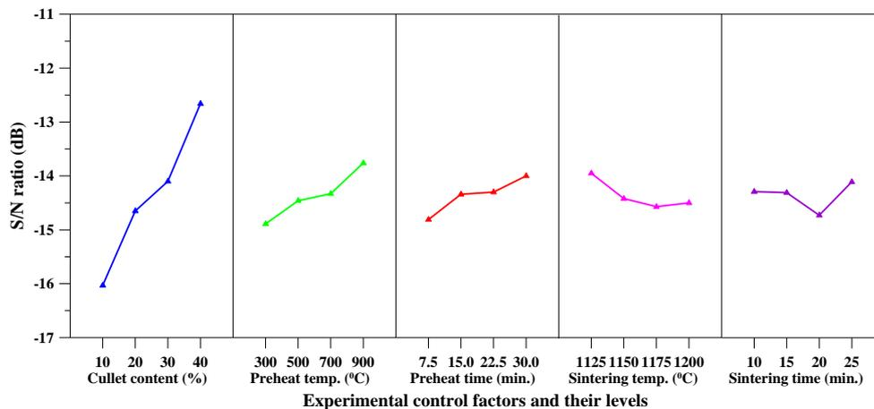
Fig. 6 S/N response graph for loss of ignition
