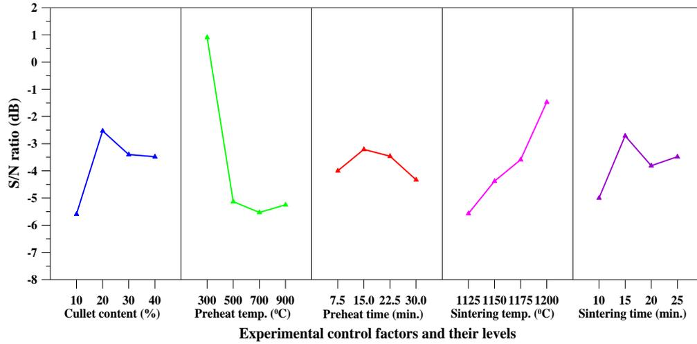
Fig. 3 S/N response graph for particle density
