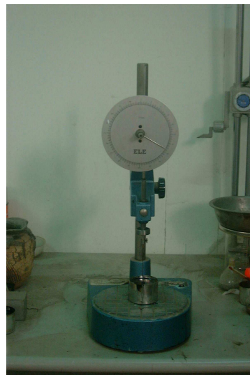
瀝青膠泥針入度試驗儀
